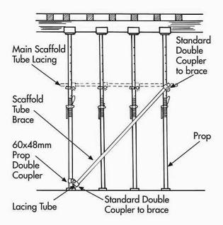
Designed & Manufactured according to the requirements of BSEN1065:1999. Adjustable props are designed to support a wide range of temporary supports for slabs & Beams and are available with or without stirrup heads.
